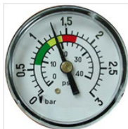
1,3 kg/cm 2 : The pressure is 0.5 kg/cm 2 more than the initial pressure, indicating that WASHING is required.
